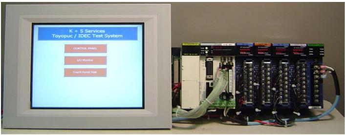
K+S Belgium is pleased to announce it's new repair capability for the Toyopuc PLC3JD system with an integrated IDEC video touch panel. This system has special I/O and touch screen programs written for it to ensure complete system testing.
